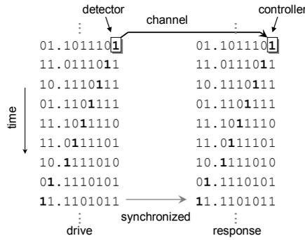
Figure 3. Communication process showing only one symbol per return communication required to sustain synchronization.
