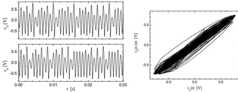
Figure 8. Drive ( $v_D$ ) and response ( $v_R$ ) waveforms for synchronization with a 2-cycle anticipation ( $\Delta t = 1.7$  ms). D is detected with  $n = 9$ , and R is controlled at  $m = 6$ .
