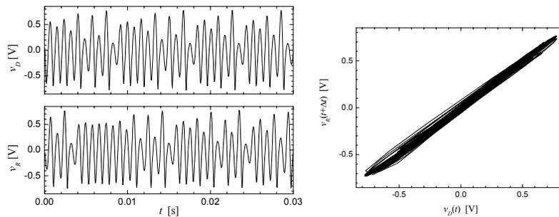
Figure 6. Drive ( $v_D$ ) and response ( $v_R$ ) waveforms measured from electronic circuits showing synchronization with an 8-cycle lag ( $\Delta t = 6.7$  ms). D is detected with  $n = 1$  bit of precision, and R is controlled at the  $m = 8$  future bit.
