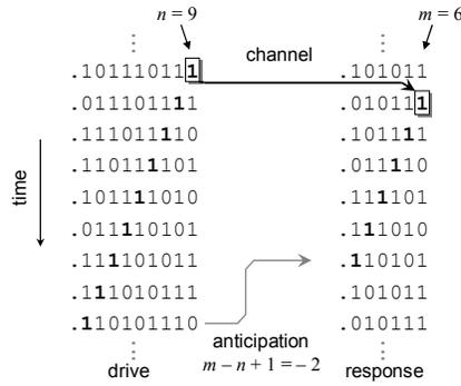
Figure 7. Lead or anticipating synchronization achieved by detecting D with  $n = 9$  and controlling R at  $m = 6$ .
