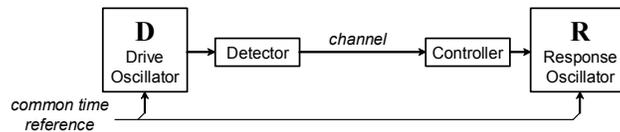
Figure 1. Drive-response configuration for investigating synchronization with unidirectional coupling.
