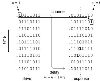
Figure 5. Lag or delay synchronization achieved by detecting D with  $n = 1$  symbol precision, and R is controlled at the  $m = 8$  future symbol.
