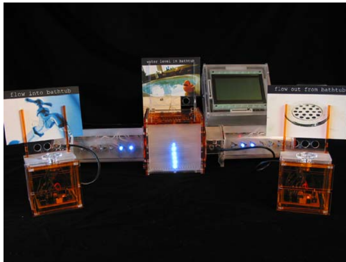
Figure. 1. System Blocks simulating water flow through a bathtub.
