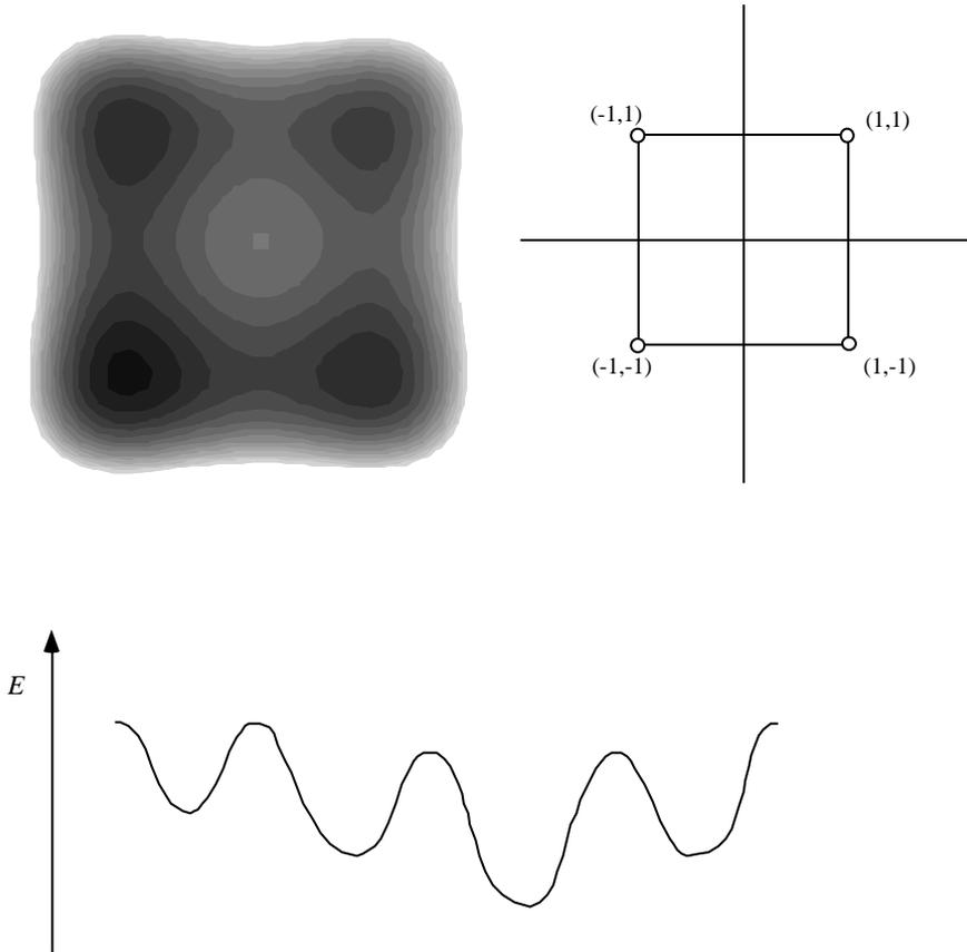
**Figure 4.3.1** Illustration of a four-state (two-spin) system formed out of two independent two-state systems. The two-dimensional energy is shown on the upper left. The coordinates of the local energy minima are shown on the right. Below, a schematic energy of the system is shown on a one-dimensional plot, where the horizontal axis goes around the square in the coordinate space of the top right figure. ■
