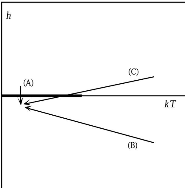
**Figure 4.5.2** Illustration of transitions in a ferromagnetic Ising model that start with different initial conditions. The transitions, indicated by arrows, are superimposed on the Ising model phase diagram. The final state in each case corresponds to having all spins DOWN. (A) is a first-order transition starting from all spins UP. (B) and (C) both start from a largely random arrangement of spins but (B) starts from a majority of DOWN spins. (C) starts from a majority of UP spins. ■
