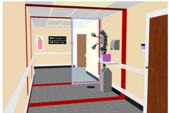
FIG. 1: A mockup of a disinfection gateway for use in inhibiting the spread of infections.
